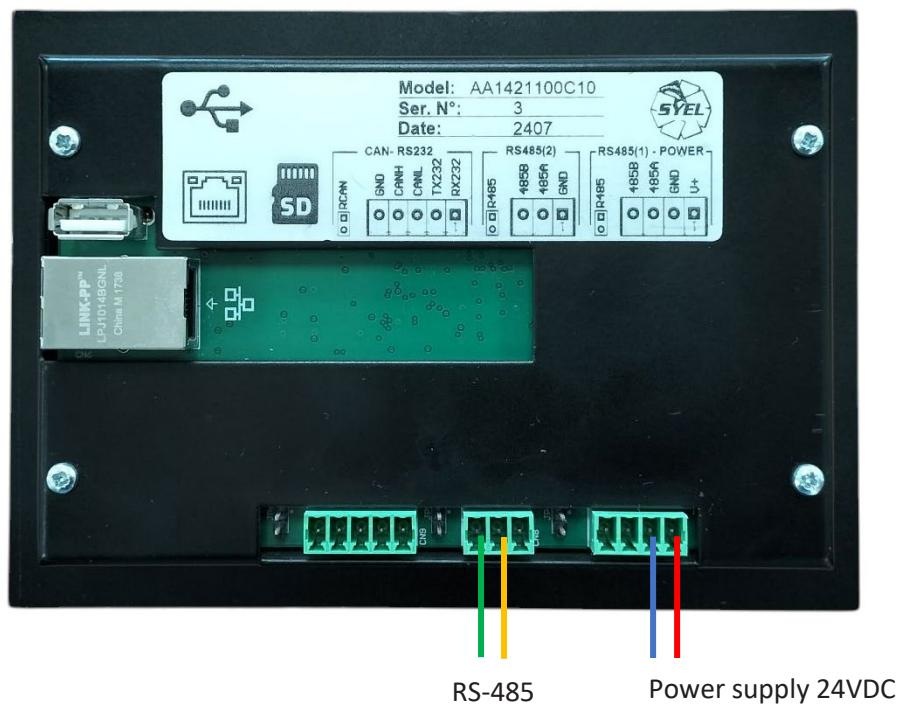
**⚠ NOTE:** The RS-485 connection can be used next to the PRIO-box on the display.
