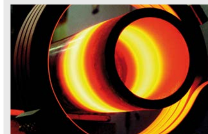
Inductively heated pipe
