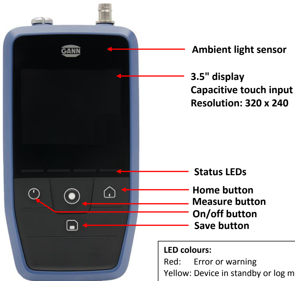
Figure 2-1: Front view of the Hydromette CH 17
