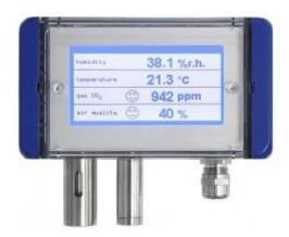
The multifunctional air quality sensor CO2-M/A measures the CO2 concentration in the ambient air in the range of 0–10000 ppm (NDIR), mixed gas VOC in the range of 0...100% based on the calibration gas, the temperature and optionally the relative humidity, absolute humidity, mixing ratio or the dew point temperature of the ambient air.
