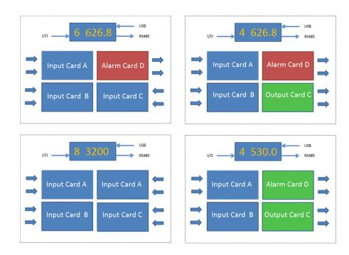
Slots of the mother board are freely selectable for input and output cards.
