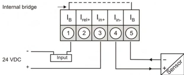
Current loop device in combination with a 3-/4-wire sensor:
