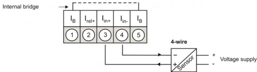
Current loop device with activated outputs 24 VDC (upto 0.4 A):
