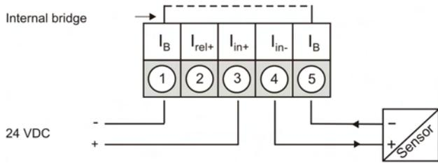
Current loop device in combination with another measuring input with low burden:
