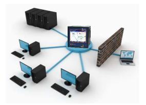
Applications in which data recorded by one device are handled by more than one person, or where the data are important in several process points, can be also implemented based on data downloading using the DAQ Manager. Several computers with an installed software can successfully download data from the same MultiCon recorder at the same time.
