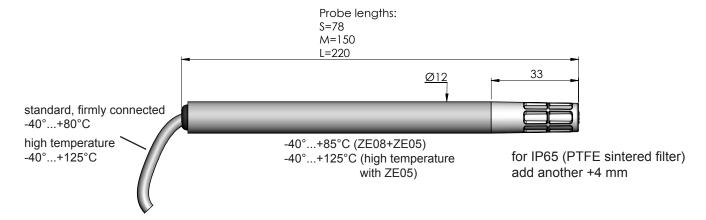
**Probe pluggable** (not possible for cable probe high temperature +125°C)
