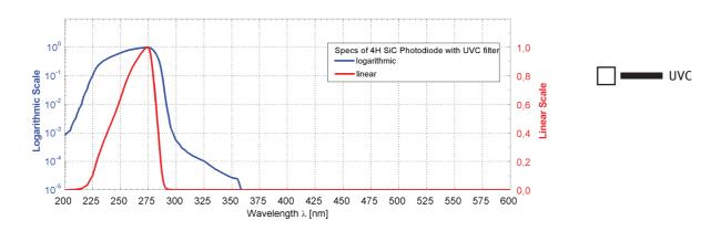
The UV-DVGW sensor is always configured with UVC responsivity according to DVGW W294-3(2006) and OENORM 5873.
