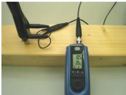
Figure 4-3 Measuring across the fibre direction with M 20
