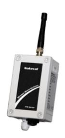
FTR970B is a radio data receiver for Nokeval MTR-series wireless transmitters. It receives and buffers the data packets that wireless transmitters have sent. It automatically recognizes the types of the transmitters, so different kinds of transmitters can be used simultaneously. Transmitters can also have different transmission intervals. FTR970B uses license free 433.92 MHz frequency band (ISM) so it can be freely used, for example, almost in whole Europe.
