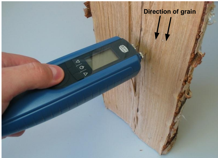
Figure 4-1 Measuring perpendicular to the grain
