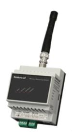
RTR970 is radio data receiver for Nokeval MTR series wireless transmitters. It receives and buffers the data packets that MTR transmitters have sent. It automatically recognizes the types of the transmitters, so different kinds of transmitters can be used simultaneously. Transmitters can also have different transmission intervals. RTR970 uses license free 433.92 MHz frequency band (ISM) so it can be freely used, for example, almost in whole Europe.
