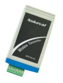
MTR264 is a battery powered, 4 channel wireless transmitter. It is housed in a compact plastic enclosure and equipped with a 6-terminal detachable screw post connector.
