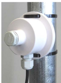
Figure 1: S-BPB Mounted to Tripod Mast
