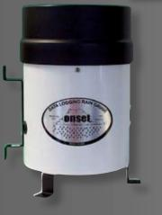
Constructed from field-proven corrosion-resistant components: aluminum housing and collector ring; stainless steel shaft and brass bearings; tipping bucket is high-precision, injection-molded, high-impact ABS plastic
