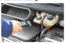
Check temperatures of engines and catalytic converters, scan ignition system problems, analyse cooling system restrictions, diagnose air conditioning systems, check tyres and brakes with uneven braking.
