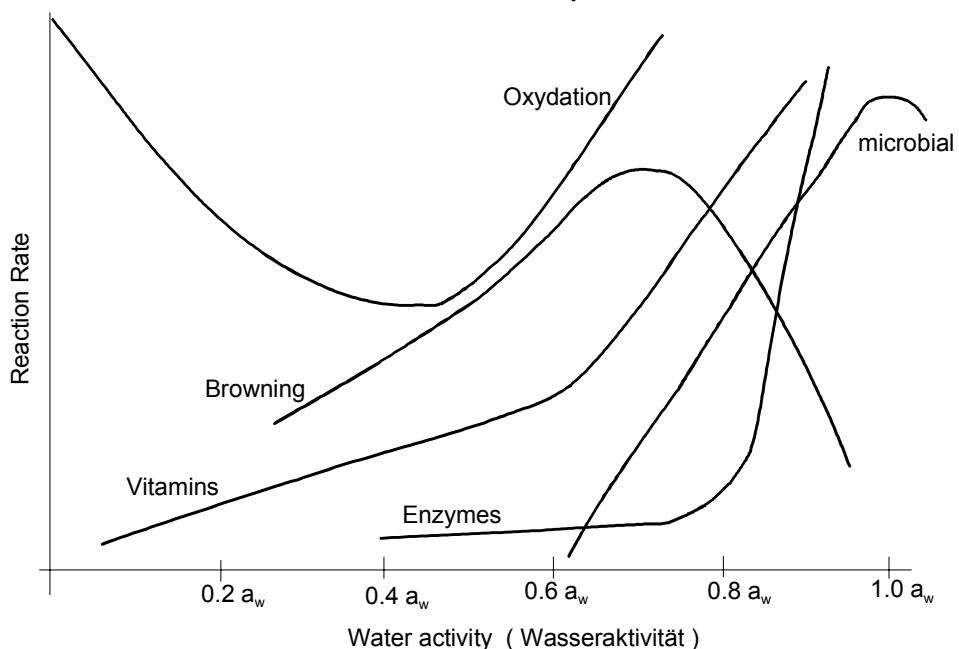
The optimisation and stabilisation of the product properties require a partially narrow upper as well as lower aw value margin. The aw – value of a product can be changed by adding of so called Humectans. Nowadays the measurement of water activity in the food industry is established in research, development, quality control and production.
