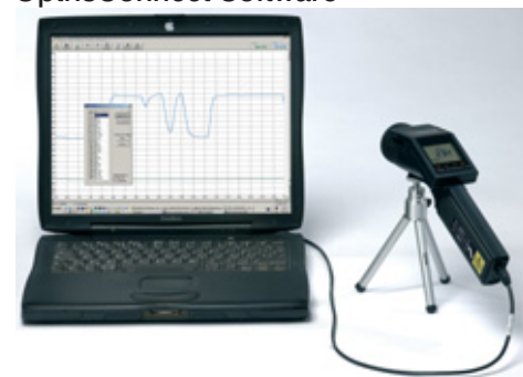
OptrisConnect oscilloscope software with 20 readings per second
