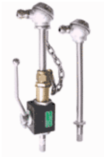
Pressure proof Humidity and Temperature Sensors in stainless steel housing for pressure up to 25 bar with ball tap exchangeable under pressure up to 10 bar
